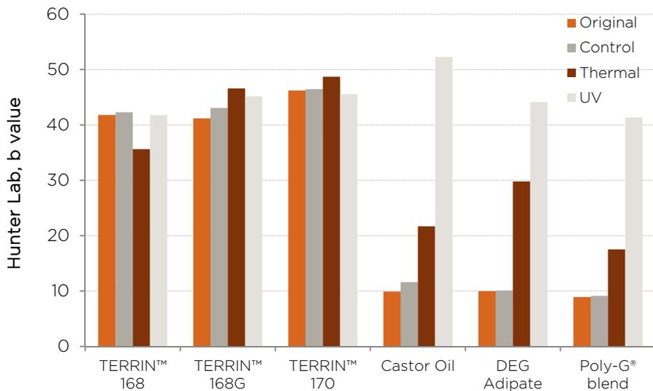
Figure 3: Hunter Lab "b" color coordinate of control (unexposed) and exposed coatings before and after testing.
