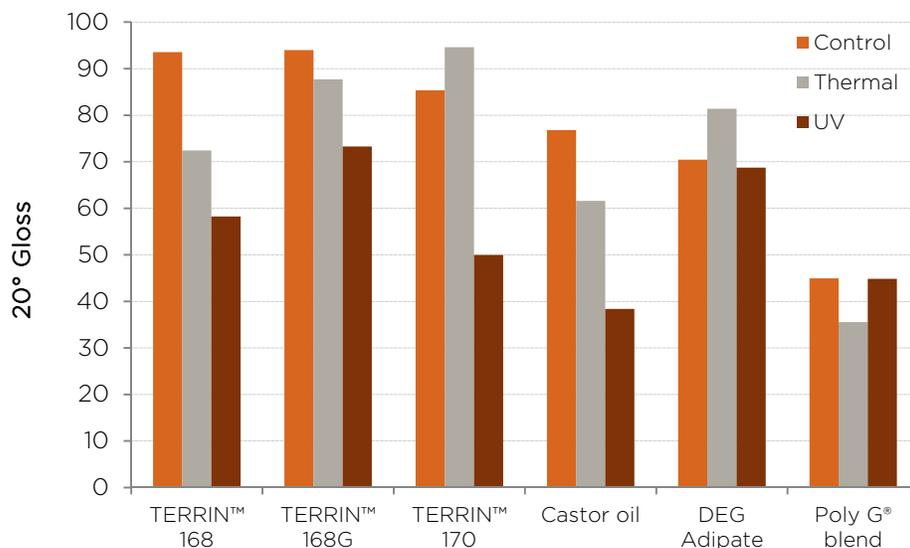
Figure 4: Gloss measured at 20° using a BYK-Gardner micro-TRI-gloss meter 200 days after coating preparation and exposure as described in the text. All samples except Poly G® blend exhibited 60° gloss > 70 and are considered high gloss.
