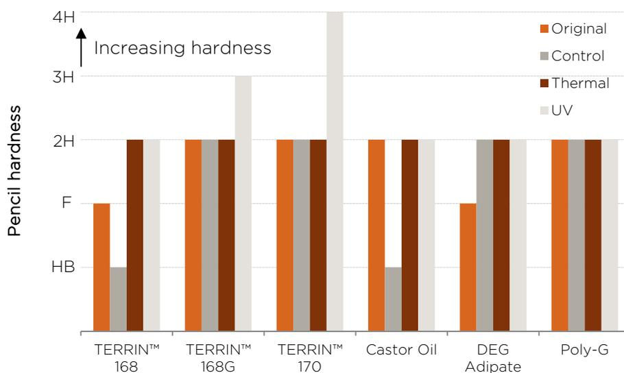
Figure 5: Pencil hardness of control (unexposed) and exposed coatings before/after testing.
